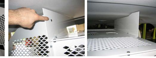
Attach ceiling filler panel to front partition using <sup>1</sup>/<sub>4</sub>" x <sup>3</sup>/<sub>4</sub>" carriage bolt and nut
